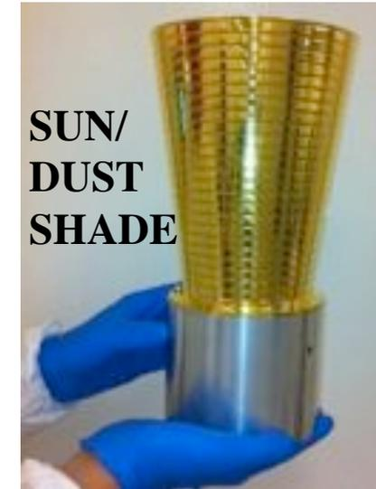
INNER CONFORMAL THERMAL SHIELD (Au-Ag coated)
